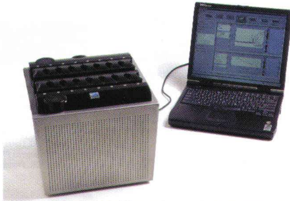
Figure 2: The portable Smart Cycler TD. Real-time PCR assays can be conducted at remote/field locations using the Smart Cycler. The Smart Cycler processing block has 16 independently-controlled reaction sites (I-CORE modules) allowing different cycling parameters to be run simultaneously.
